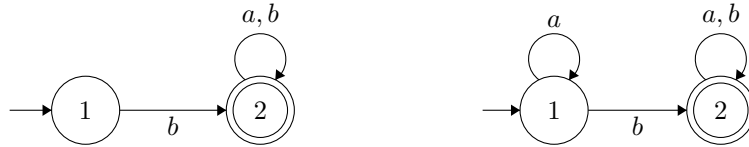
Figure 2: Different minimal ROWJFA accepting the language \{w \in \{a, b\}^* \mid |w|_b > 0\} .
