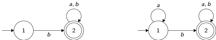
Figure: Different minimal \text{DFA}_{\text{reg}} accepting the language \{w \in \{a, b\}^* \mid |w|_b > 0\} .
