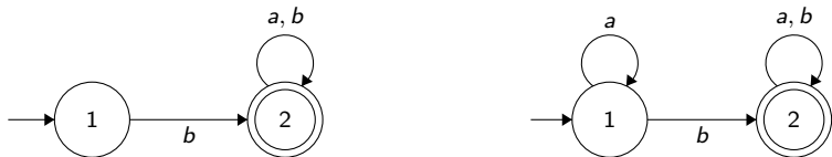
Figure: Different minimal \text{DFA} accepting the language \{w \in \{a, b\}^* \mid |w|_b > 0\} .
